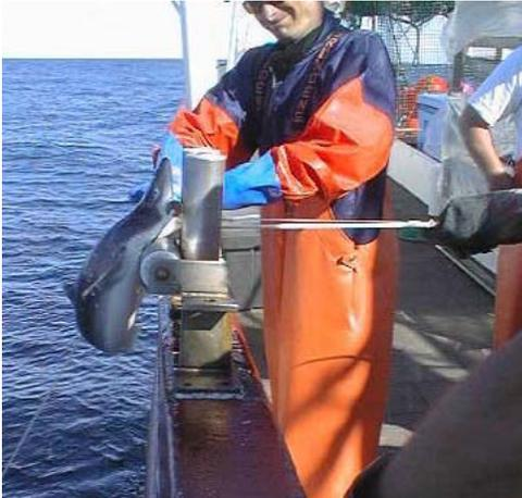
Figure 2. Stainless steel rollers installed on board the F/V Isabel S. One of the many dogfish caught in July 2000 being snubbed from the longline.
