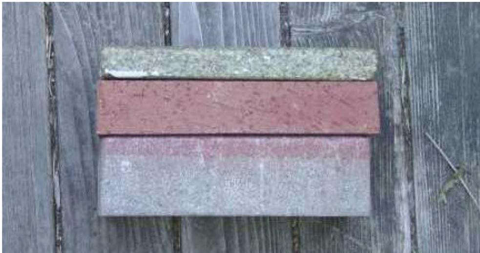
Figure 11 - Thickness of glass (top), brick (middle) and concrete (bottom) pavers
