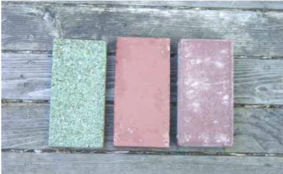
Figure 12 - Glass (left), brick (middle) and concrete (right) pavers
