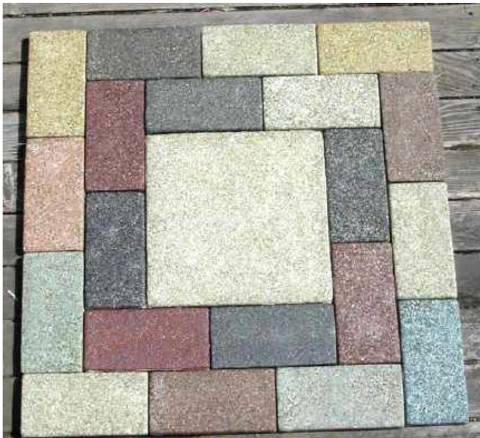
Figure 13 – Display of 4” x 8” and 12” x 12” colored glass tiles
