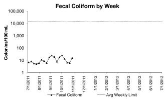
In October, all permit conditions for Fecal Coliform were met. Fecal Coliform is an indicator of the presence of pathogens. The levels of these bacteria after disinfection show how effectively the plant is inactivating many forms of disease-causing microorganisms.
