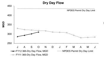
October's Dry Day Flow is the average of all dry day flows for the period from 11/1/2010 to 10/31/2011. The Dry Day Flow for September was 310.3 MGD, well below the permit limit of 436 MGD. Dry Day Flow is calculated by averaging influent flows over the previous 365 days during dry weather.
