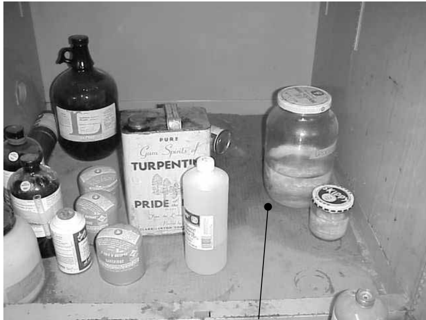
Base Of Flameproof Cabinet Covered with Cardboard, Note Stain
