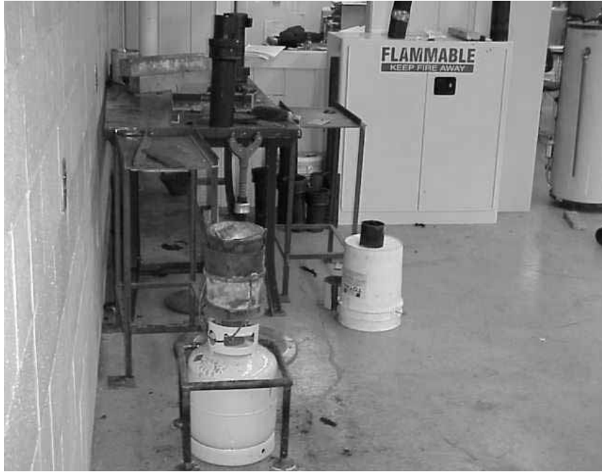
Ingot Melting Using Propane Tank, Note Flameproof Cabinet
