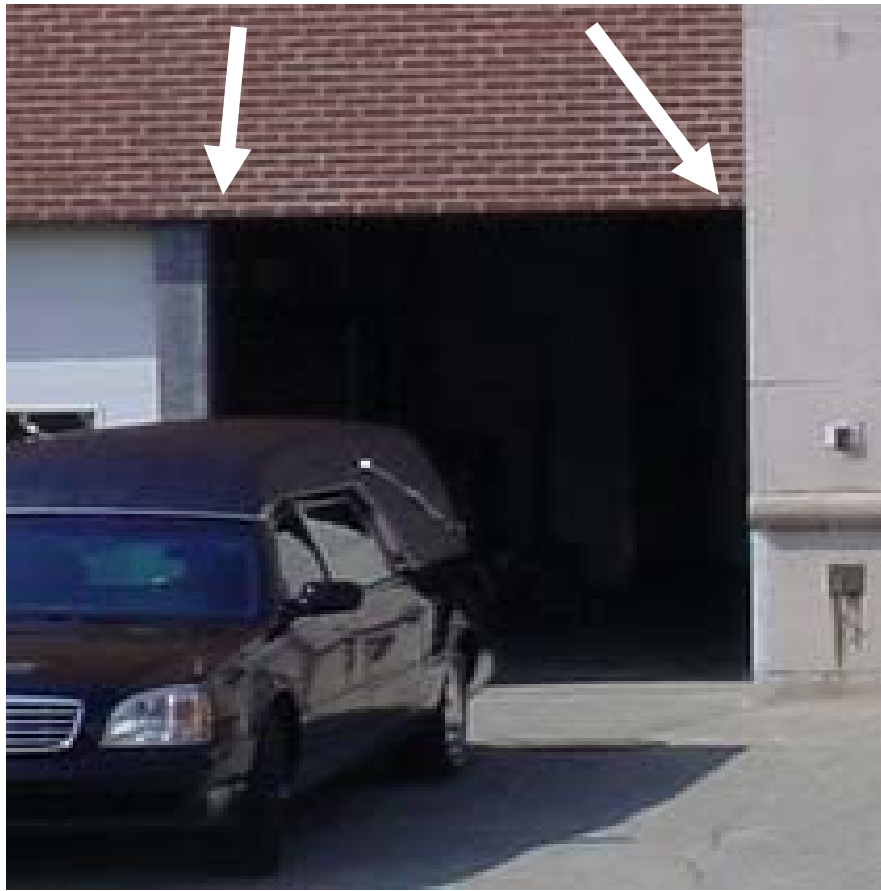
Location Where Strip Door Should Be Attached on Outside Of Building (see arrows)
