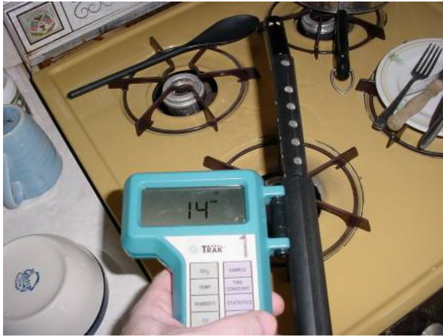
Carbon Monoxide Measurement in Kitchen with Gas Stove Combusting Fuel
