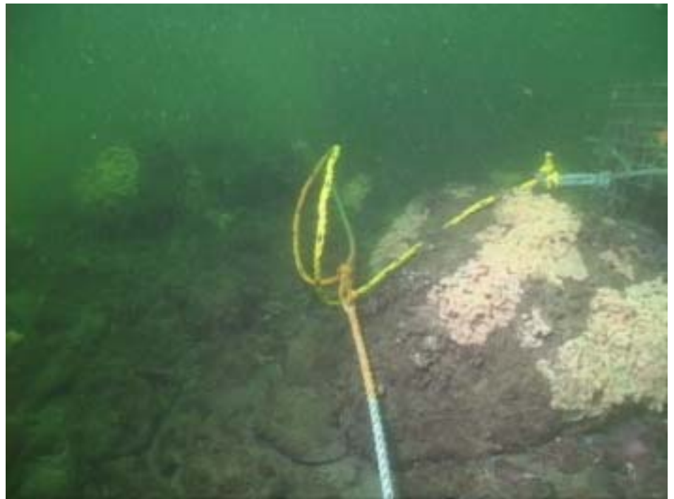
Figure 6. Use of floating line gangions had no effect on the measured height of the neutral buoyant mainline.
