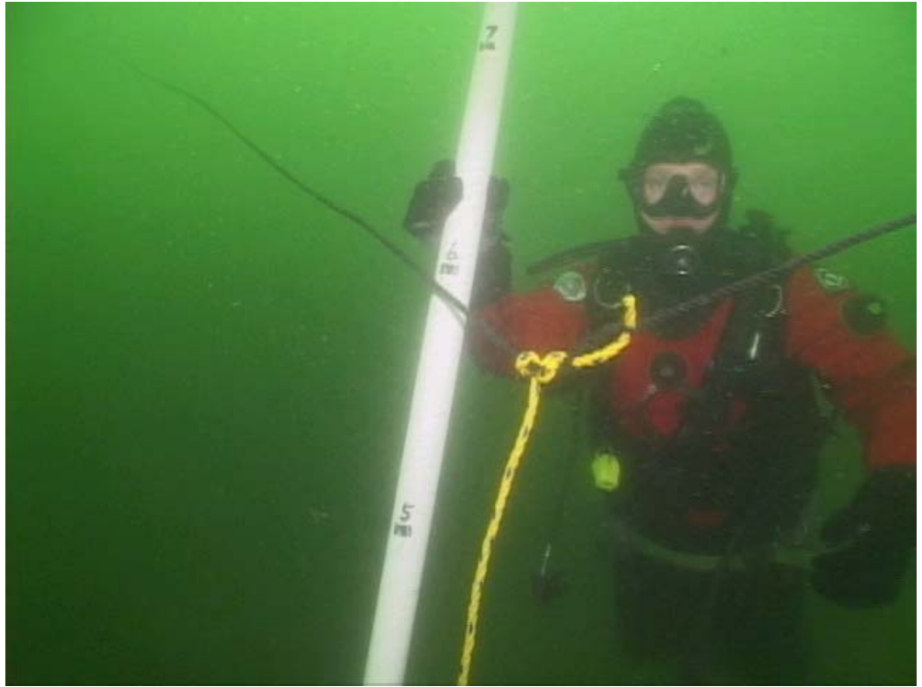
Figure 2. DMF Diver Bob Glenn measuring the maximum height of the gangion (~5.5 ft) on a trawl rigged with all floating groundline.
