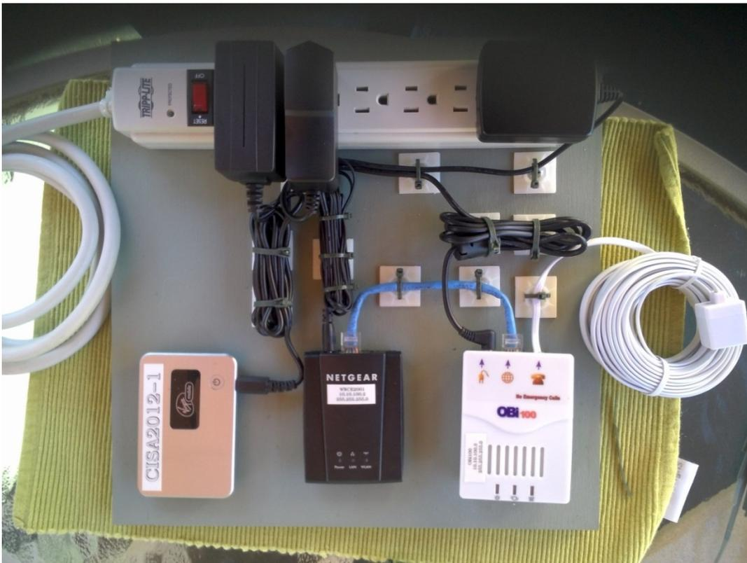
*Connectivity board designed to enhance connections for processing HIP and SNAP transactions.*
