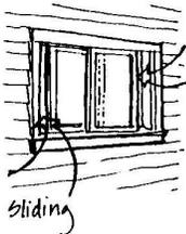
**Materials.** Vinyl- or aluminum-clad wood windows are ideal for ease of maintenance. Wood windows require a high level of maintenance (periodic painting) and are only acceptable when required for historic preservation projects. Avoid using unprotected aluminum near salt water. Consider fiberglass windows.
