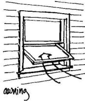
Awning and casement windows are an acceptable alternative; they are convenient for hard-to-reach areas such as over a kitchen sink. Awning windows do a better job of keeping out the rain than casements. For barrier-free units, awning and casements may be desirable so that residents can supply their own motorized window operators. Be sure that ground floor windows that swing out are located out of the way of footpaths.
