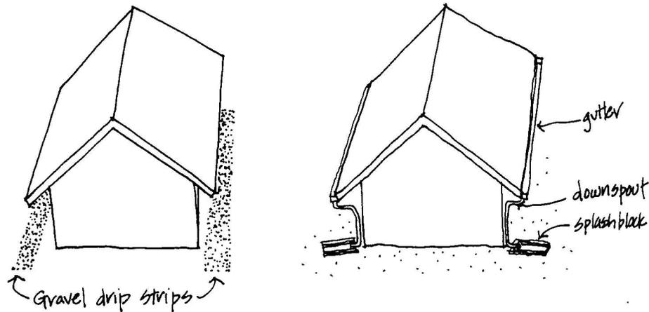
**Gutters.** Gutters add to initial construction cost and require routine inspection for damage and routine maintenance to keep them free of leaves and debris. Gutters are necessary to protect doorways, walkways, landscaping, and other areas from the splash of rainwater but may not be required where deep roof eaves carry water away from the building. Provide screens on gutters to prevent them from getting clogged.
