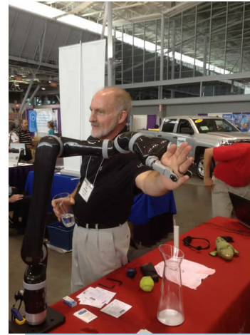
Demonstrating the grip of the Jaco robotic arm ( http://kinovarobotics.com )
