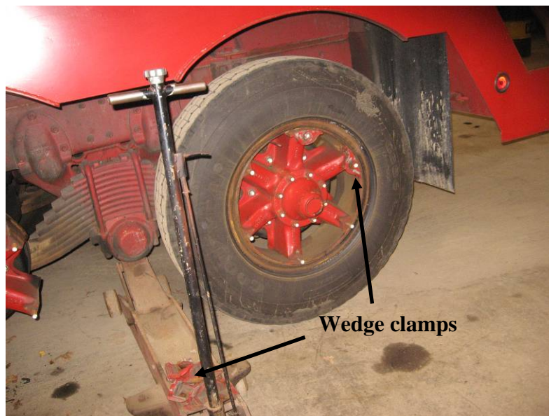
Figure 3 – Demountable rim wheel with wedge clamp
