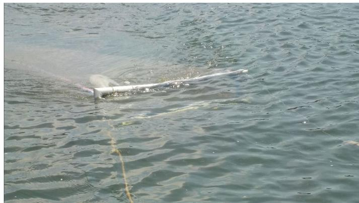
A manta net deployed in the Merrimack River to collect microplastics for analysis. (Photo: Peter Phippen)
