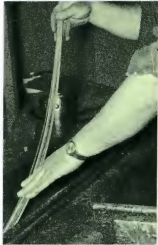
9 Rod section dipped in hot glue.
