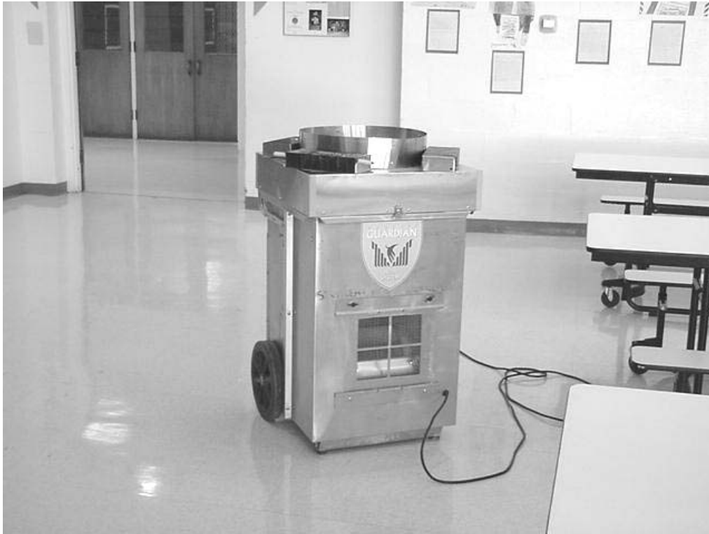
Exhaust Fan Equipped With HEPA Filtration
