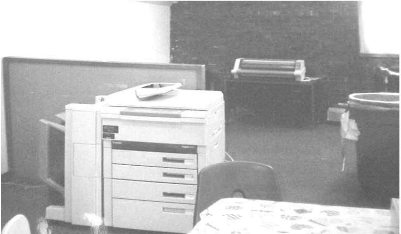
Photocopier and Lamination Machine Noted in Teacher's Lounge Note No Mechanical Exhaust Ventilation is Provided in This Area
